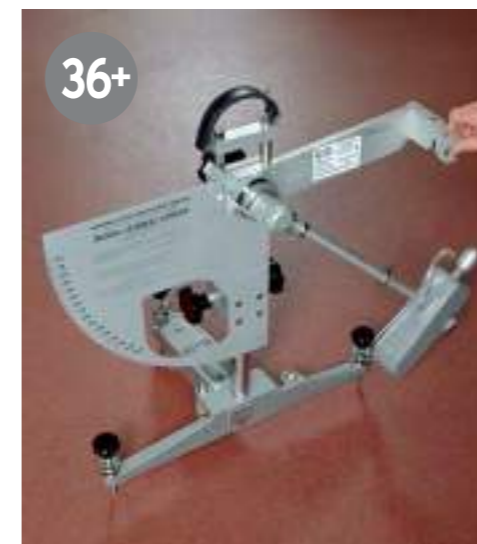
RRL Pendulum Co-Efficient of Friction Test
